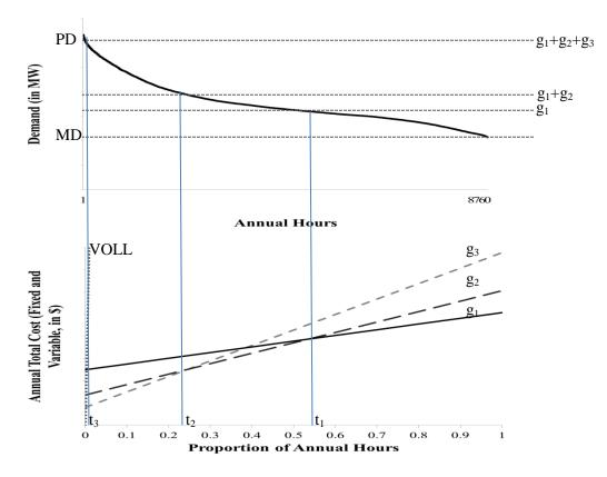
**Figure A1:** (Top) Load Duration Curve - Number of hours per year that load is at or below each demand level; (Bottom) Generation Screening Curve – Fixed and variable cost of operation
